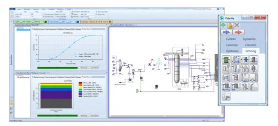
Aspen HYSYS Petroleum Refining provides users with simplified and rigorous unit operations in the palette featured above to manage model complexity.
